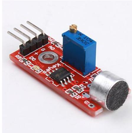
**Figure 1. Arduino board compatible microphone sensor**
