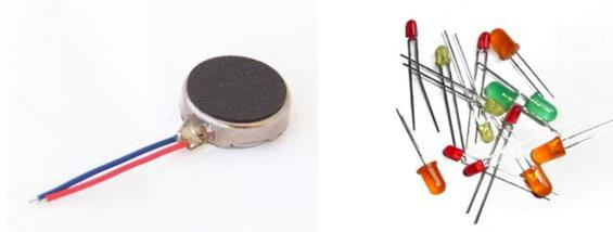
**Figure 3. Output: Vibration motor and LED light**
